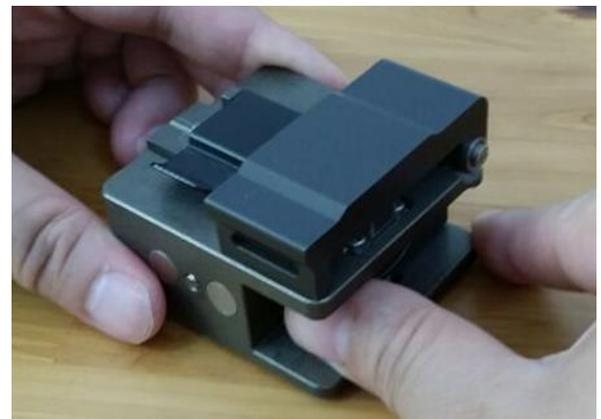
2.7.5 Hold the cutter by left hand and open the big clip by right hand and remove the fiber chips to put them in fixed containers.
